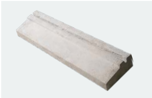
Sunk, weathered, throated and grooved, throat 12mm wide and 12mm from front edge
